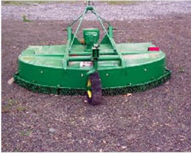
3. Some reflective markers (and some red/amber lights are working if equipment is over 13 feet wide) are broken, missing, or dirty.
