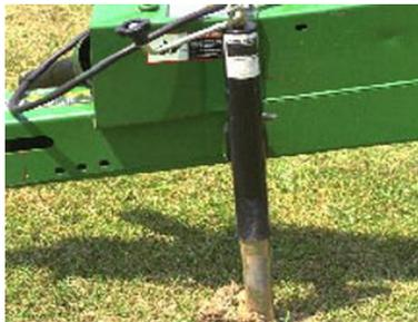
5. Equipment/machine has a jack stand. Jack stand is in good condition, has a good hand crank, can be secured in an up position when not needed.
