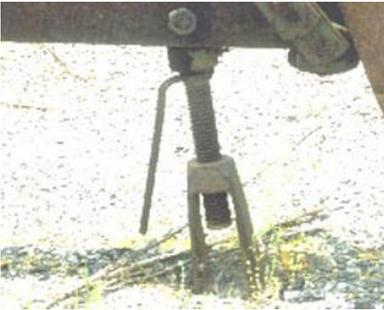
3. Equipment/machine has a jack stand. Jack stand is bent, doesn't sit level on the ground, hand crank is damaged or missing, secured in an up position with a makeshift latch/tie.
