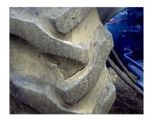
3. Tread is wearing, a few sidewall cracks.
