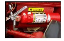
3. BC type fire extinguisher with at least a 5 pound capacity is mounted on the tractor.
