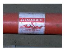
5. Warning decal(s) are mounted on PTO shield or on implement hitch below shaft where they are easily read; includes pictogram.
