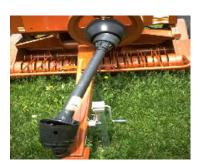
5. Driveline shaft shield is in place, is in good condition, and it can easily rotate by hand. Chain prevents shield from rotating.
