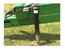
Equipment/machine has a jack stand. Jack stand is in good condition, has a good hand crank, can be secured in an up position when not needed.
